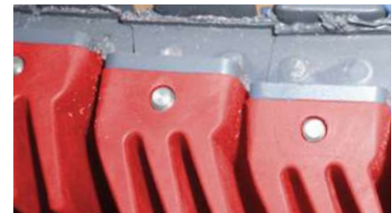
Melted flight material
