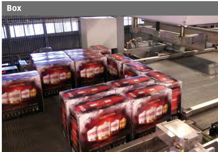
Box LBP: basically for accumulation GT: basically for inclines/declines and stop-divider applications
