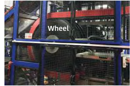
Exceeded pv-limit at chain
